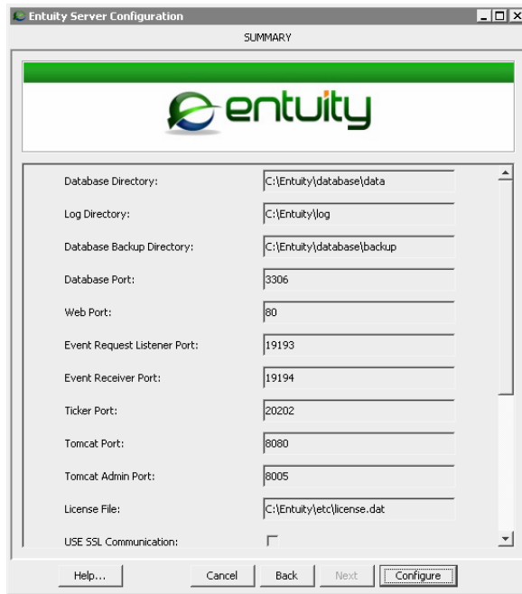
Figure 23 Final Configuration Check
